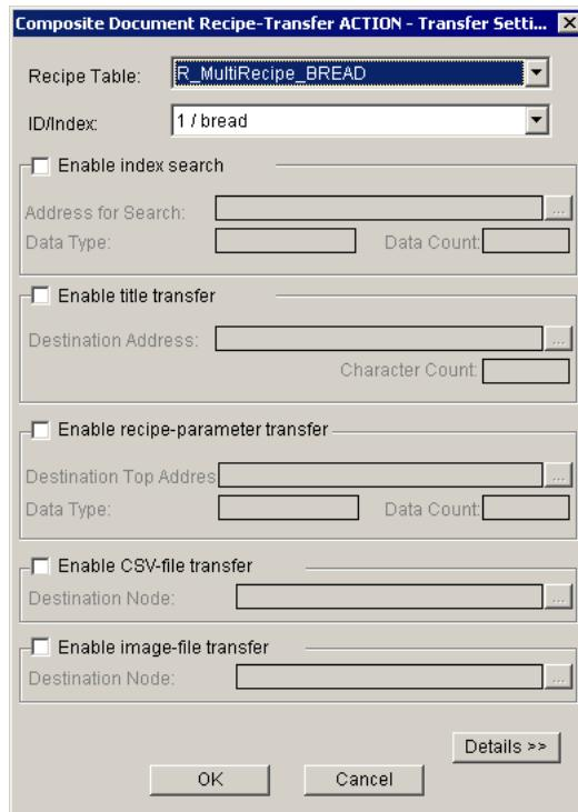
10 Select the composite data to be transferred from the list of the composite data stored in the selected table in [ID/Index], and click [Details]. Then, details of the selected composite data are displayed.
