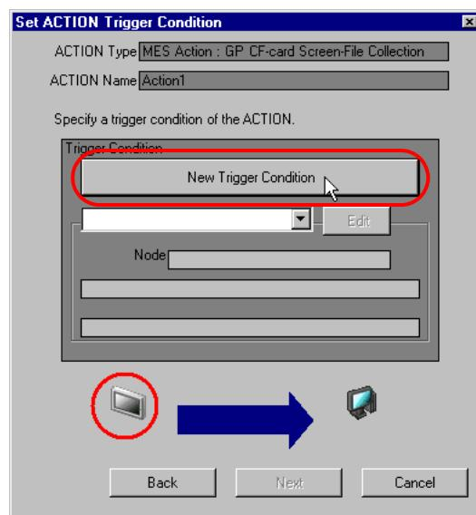
**12** Specify a trigger condition name and node name. Then, specify a trigger condition in the [Condition 1] tab.
