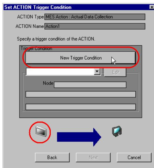
14 Specify a trigger condition name and node name. Then, specify a trigger condition in the [Condition 1] tab.
